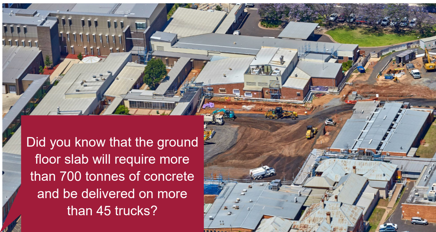
This aerial photo taken in November 2018, shows a portion of the footprint for the new three-storey clinical building. The structure will be built in stages (starting with the back of the building and working to the front) to minimise disruption to services.
